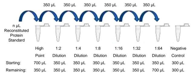
For samples of unknown protein concentrations, serial dilute the experimental sample using Assay Diluent to determine range of detection and acceptable dilutions. Shown below is a diagram illustrating a 10-fold serial dilution on a given Sample of Interest.
