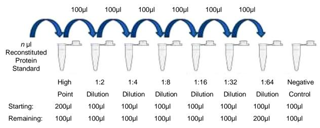
For samples of unknown protein concentrations, serial dilute the experimental sample using Sample Diluent to determine range of detection and acceptable dilutions. Shown below is a diagram illustrating a 10-fold serial dilution on a given Sample of Interest.
