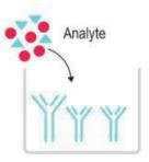
1. Add 100µL standard or sample to the wells. Incubate for 90 min at 37°C
